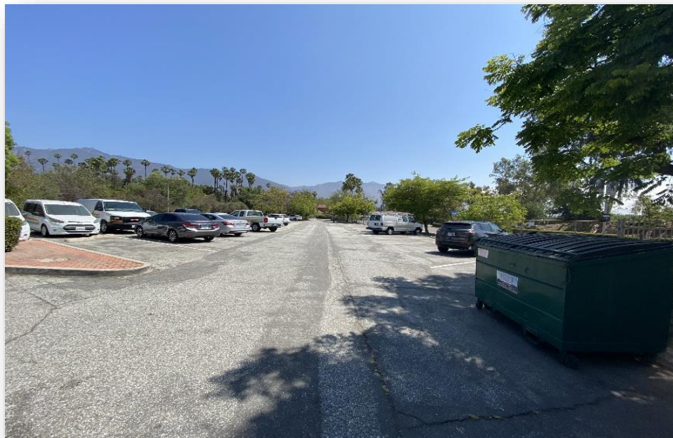
A view of a parking lot with no identified path of travel, and no signage directing users to an accessible entrance
